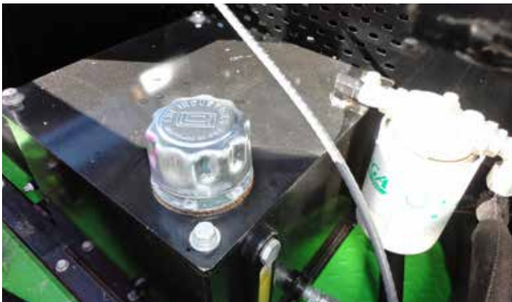
15 Gal. Hydraulic Tank & Filter System with Sight Gauge
