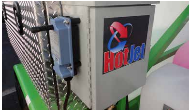
Nema 4 Control Box & Remote Control
