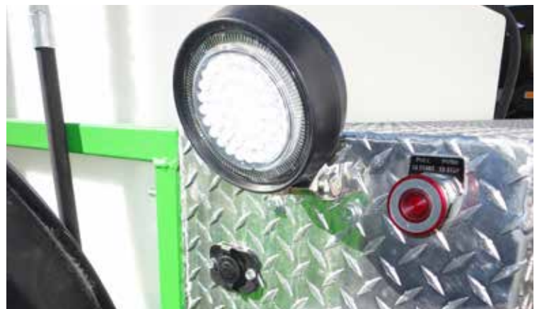
Rear L.E.D. Lighting w/Safety Shut Off Control
