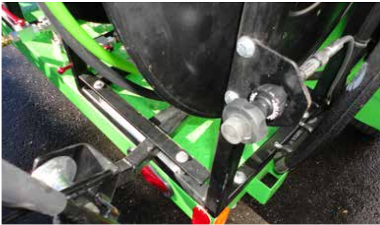
Rear Throttle Control & 120° Hose Reel Guide
