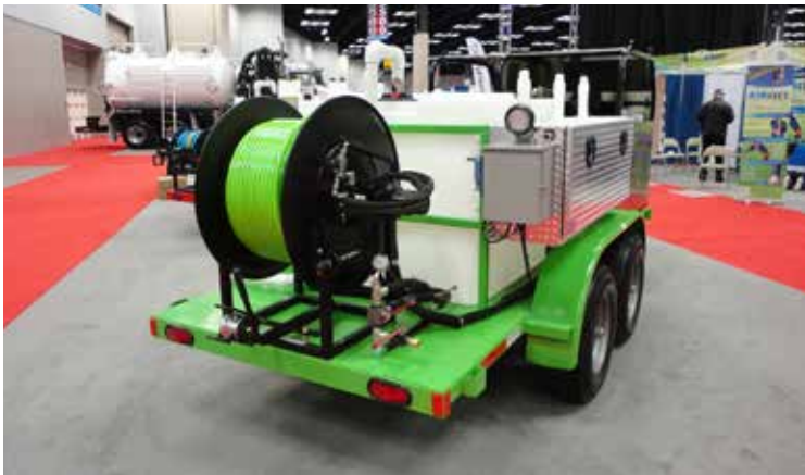
Reel Options... 500' x 1/2" Hose or 500' x 3/4" Hose for 40 gal. GPM or Both
