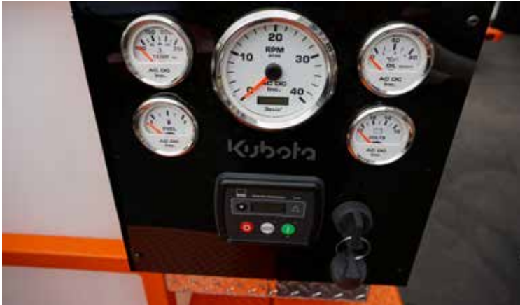
Deep Sea Electronics for Engine Control
