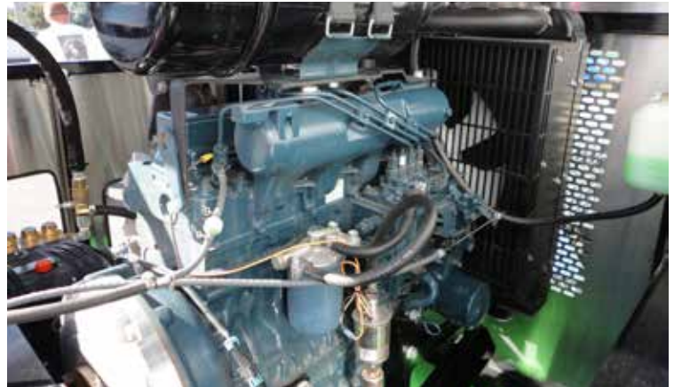
Easy Access to All Filters (Air, Fuel, & Oil) & Injection Systems
