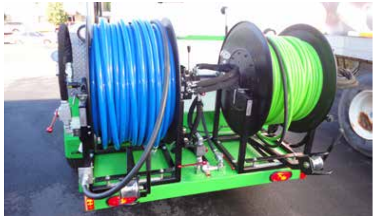
Reel Options... 500' x 1/2" Hose or 500' x 3/4" Hose for 40 gal. GPM or Both
