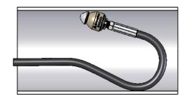
SAFETY! If the WV is being used in pipes larger than 4 inch diameter, a rigid stinger should be installed between the tool inlet and the hose end; otherwise the tool can turn around and come back toward the operator, causing serious injury or death.
